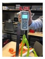
The harness strap (Lo=6in) deformed 0.07in, which is less than 10% of the original length.
