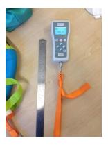
The tow strap (Lo=10in) deformed 0.1in under 170N, which is less than 10% of original length.
