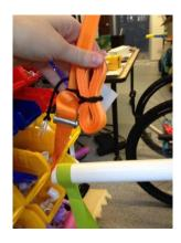
This was solved by tying up the loose end, which now measures 2.5", less than 3", and so passing the test. The instruction manual with direct parents to trim the end ~3ft after the desired length and zip tie the remainder together so it is not accessible to children.
