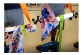
The only area with significant pinching was the easy release buckle on the tow strap connecting harness to swivel. The team covered it with a cut sock so the buckle was not acceptable to children.
