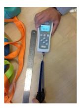
The bungee cord (Lo=3in) did not pass the test, as it deformed over 1in with only 60N of force. The team switched to using nylon rope on the bearing connection since it deformed the least of all elastic materials.
